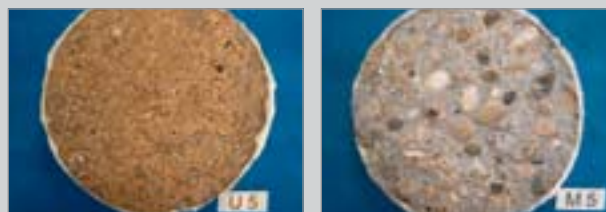
Picture 2: Difference between concrete cores (left side with Zemdrain®, right side without Zemdrain®), after 56 freeze/thaw cycles.
